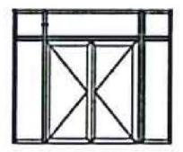
Doorsets incorporating side lights and/or fan lights may be constructed using a 'T-Bar' or 'Split Coupled Joint' method. Please see the data sheet for further details.
