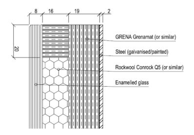
The above construction may be used in the "CW50 – FP" Curtain Walling for applications of up to 60 minutes integrity and 60 minutes insulation. The steel face, of the construction, must be oriented to the fire.
